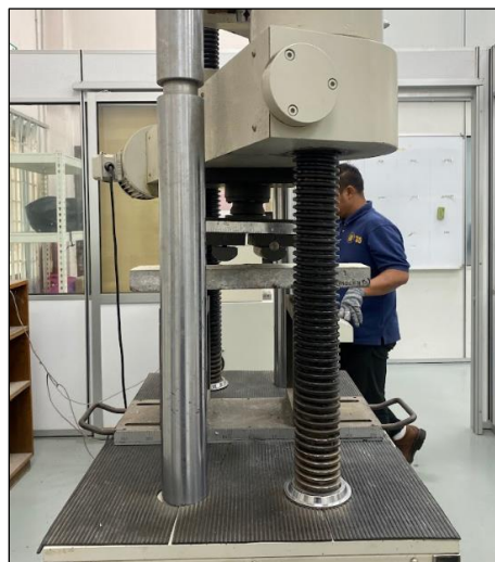
Figure 5. Set-Up for The Flexural Strength Test
