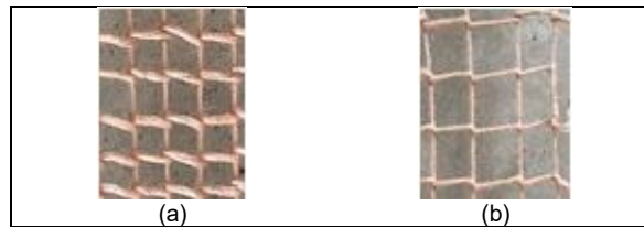
Figure 2. Bamboo Textile Used in Strengthening of RC Slabs (a) 10 x 10mm (b) 20 x 20mm
