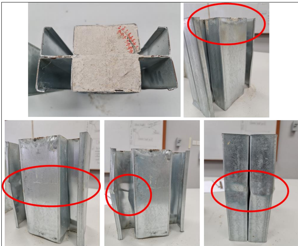
Figure 9. The Failure Mode of The BCFS2 Specimen
